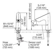
■Mounting deck thickness: 1/4" (5 mm) - 2" (50 mm)
